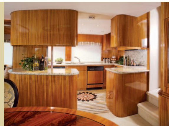
HIGH TECH Pre-finished flush-filled panels allow Hatteras craftsmen to build cabinetry that is finished to perfection before it ever gets installed on the boat.
